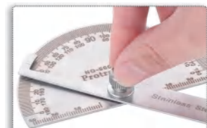
1. Adjust the required angle of the logpoint and tighten the screw
